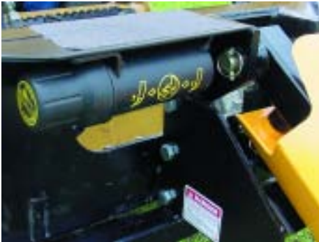
Extra large step with non-skid for entering and exiting skid loaders and owners manual canister so the manual stays with the unit at all times
