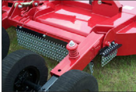
Each axle arm has a strategically placed spring cushion to absorb shock loads near the wheels.
