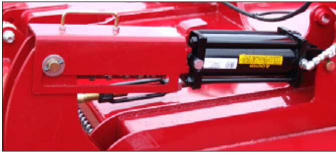
The transport lock-up device is easily positioned to take the load off the hydraulic cylinder rod during transport.
