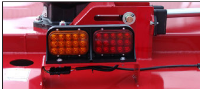
Highway lights are standard equipment. Lights provide flashing and turn signals.
