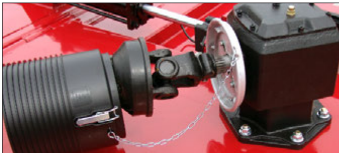
The quick detach shields allow easy access to the driveline clutch and grease fittings.
