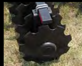
Notched discs for maximum cutting action
