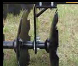
Bearing hangers reinforces with gussets
