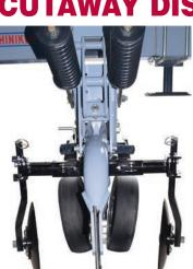
Quick and easy pin adjustments permit 10 horizontal and 14 vertical settings.
