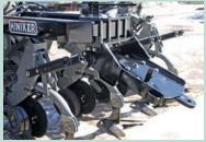
Telescoping trailer hitch provides easy hookup to fertilizer tanks. Hitches are also available for cultivators equipped with lift assist wheels.
