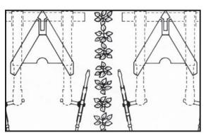
In crops as small as 3" the wheels are set aggressively with the leading edge spaced as close to the row as necessary to remove weeds but, WITHOUT the root pruning damage common to discs.
