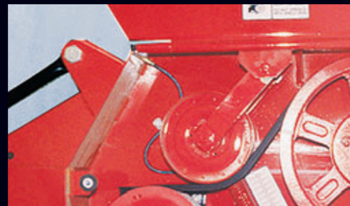
Matched "C" section belts provide extra power transfer reserve and minimum slippage. 8 inch diameter spring loaded backwrap idler extends belt life and is easily adjusted with just a screwdriver.
