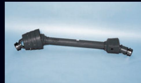
Category 5 plus constant velocity (C.V.) P.T.O.'s are standard on all trailing units. This eliminates driveline knocking and the need to disengage P.T.O. on short turns. An overrunning clutch is included to protect tractor P.T.O. during shutdown.
