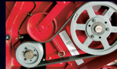
Multiple groove, banded belts deliver maximum horsepower without slippage. Spring loaded backwrap idler is easily adjusted with just a screwdriver.
