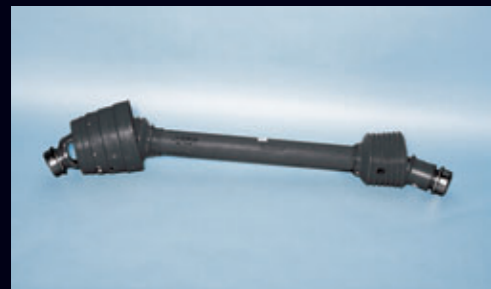
Category 5 plus constant velocity (C.V.) P.T.O.'s are standard on all trailing units. This eliminates driveline knocking and the need to disengage P.T.O. on short turns. An overrunning clutch is included to protect tractor P.T.O. during shutdown.
