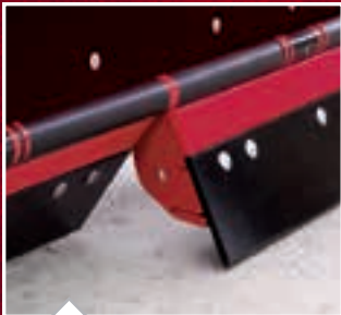
High-clearance split trip-edges operate independently of one another, reducing stress and twisting forces on the plow.
